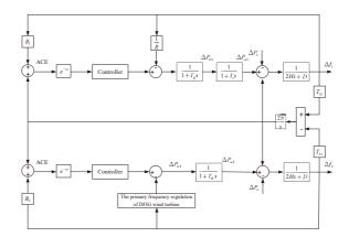
Fig. 3. The two areas frequency regulation dynamic model of AGC with DFIG turbine  $% \left( {{\rm DFIG}} \right)$
