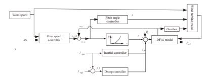
Fig. 1. The active power control model of DFIG wind turbine
